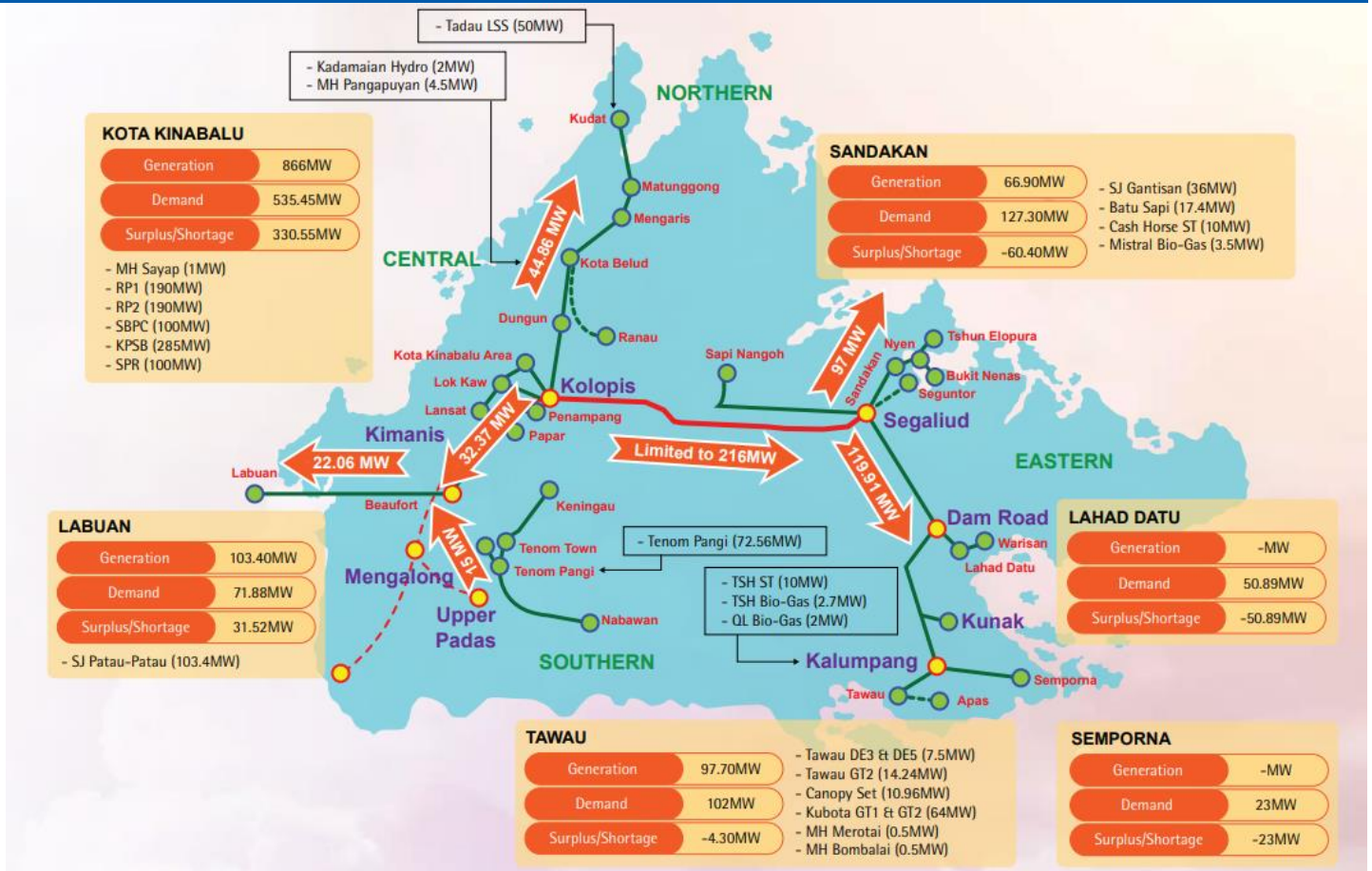
Figure 9: Kota Kinabalu's electricity surplus of 330MW vs shortages over at the east grid
