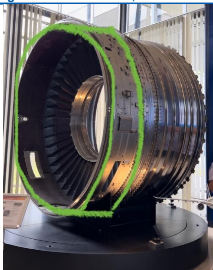
Figure 3: Area highlighted is the rear case, assembled into a fan case
