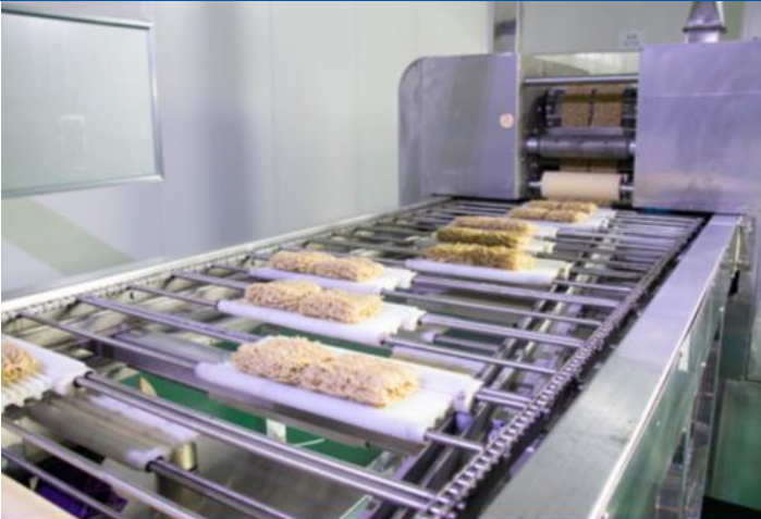
Figure 7: Noodle production line – cutting and sorting
