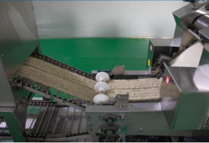
Figure 6: Noodle production line – dough pressing and forming
